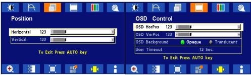
Push "Up" or "Down" button to select between "Horizontal" or "Vertical" then push "Select" Use "Left" or "Right" button to adjust
